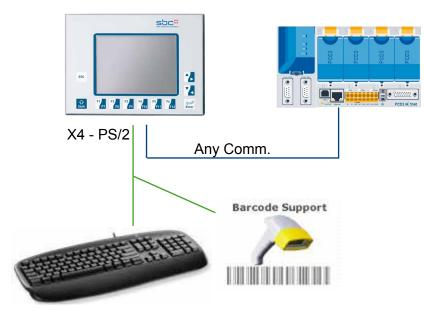
The only thing you have to do is configure which keyboard country type or Barcode reader you have at disposal. For this, just go in the Setup Menu below Keyboard and choose one of the following PS/2 Keyboard Layout in the list box.
