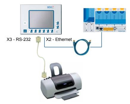
The communication speed is limited to max 115'200 bauds on RS-232 (X3) and is standard to 10/100 Mbps on Ethernet (X2).
