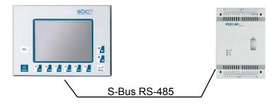
This RS-485 S-Bus connection is foreseen to be used between our PCD7.D4xx and PCD3.M3020, PCD1.M125/M135, or PCD2.M150 where «less fast» communications are acceptable.
